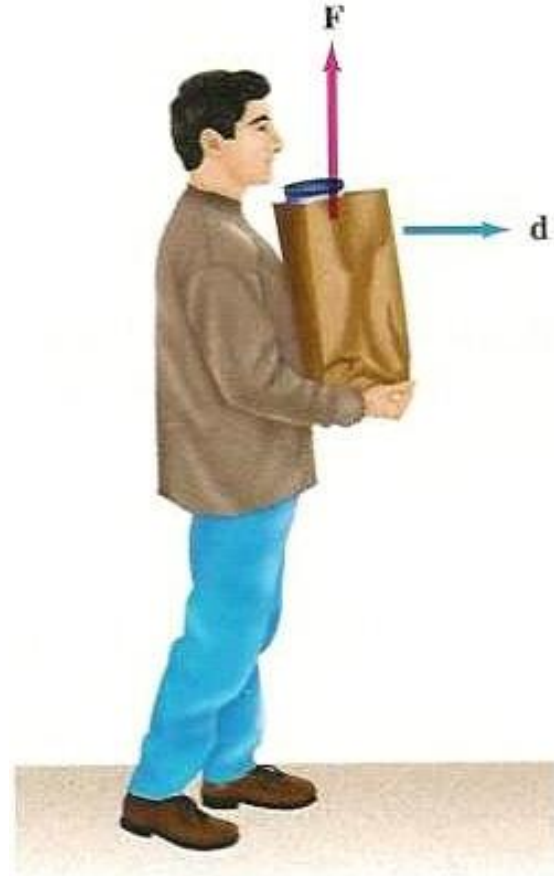
FIGURE 6-2 Work done on the bag of groceries in this case is zero since F is perpendicular to the displacement d .
